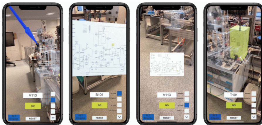
Figure 1.1: "Example functionalities in augmented reality user interfaces for digital twins. From left to right: a) indicating the position of a not-visible component. B) positioning of virtual functional diagrams in the room c) placing functional diagrams as two-dimensional user interface elements on the hand-held screen and highlight components on them. D) highlighting of requested plant components directly with a visual overlay." [8]
