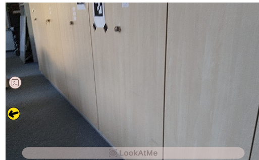
Figure 3.8: If the camera turns away from the image plane, a tiny arrow is displayed on the screen edge and the LookAtMe button is greyed out
